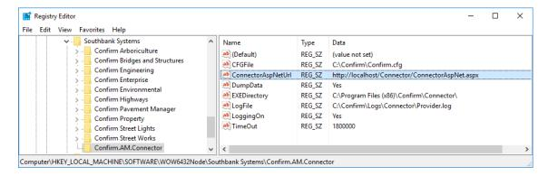
Double check that the CFGFile and LogFile settings are correct and the latter should point to a directory the Application Pool's user has write access to.
