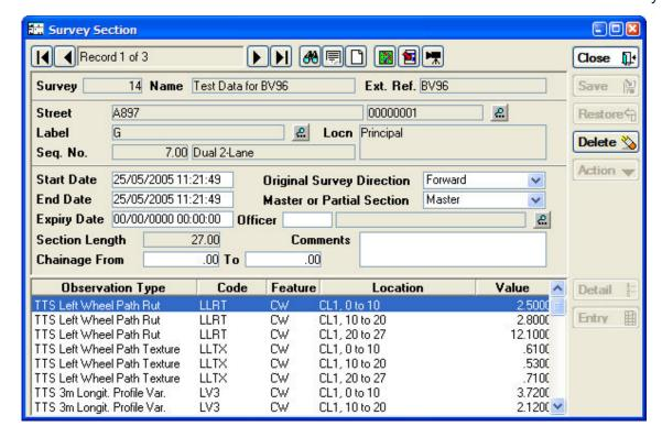
To enter new network sections, click on the Clear/New button, then choose the section you require, either by typing in entries for one or more of street, label and sequence number, or using the Pick buttons. When the using the Pick buttons it is recommended that the Label Pick button is used as this presents a filter form on which the streets can be filtered as well. If the Street Pick button is used instead, the location still has to be filtered on a separate screen later.
