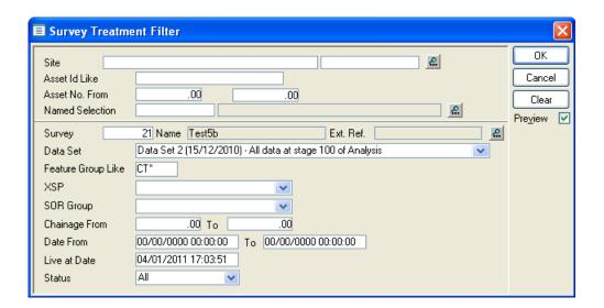
The bottom section is where the source of data is selected. The Survey and Data Set details are mandatory. The Feature Group Like refers to the Feature Group of the Survey Observations.
