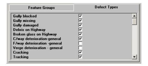
It is possible to associate Defect Types with the current Observation Type so that when this Observation Type is entered in the Defect screen the selection of Defect Types is limited to those checked here. This restriction will be applied when raising Defects directly in Confirm and when using ConfirmConnect®.
