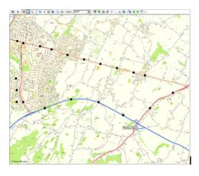
Driven survey - at constant speed the gaps are consistent
