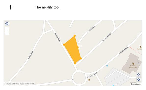
With the modify tool the user can move points, add points or delete points. To move a point the user can click and then drag it. A new point can be added by hovering over a line until a new point appears and then clicking. To delete a point the user can hover over an existing point and single click.
