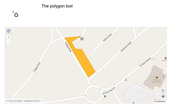
To draw a polygon single click on the map to plot a start point, and as the mouse moves a line will appear that follows it. To plot a new point on the polygon the user can single click again. Repeat this action for as many points as are required and then single click on the last plotted point to close the polygon.
