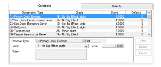
The current Condition Grade and Score for the currently highlighted Observation Type will also be displayed. Where the Observation Type has been assigned, but not graded yet, the Condition Grade will be the "NA" grade.
