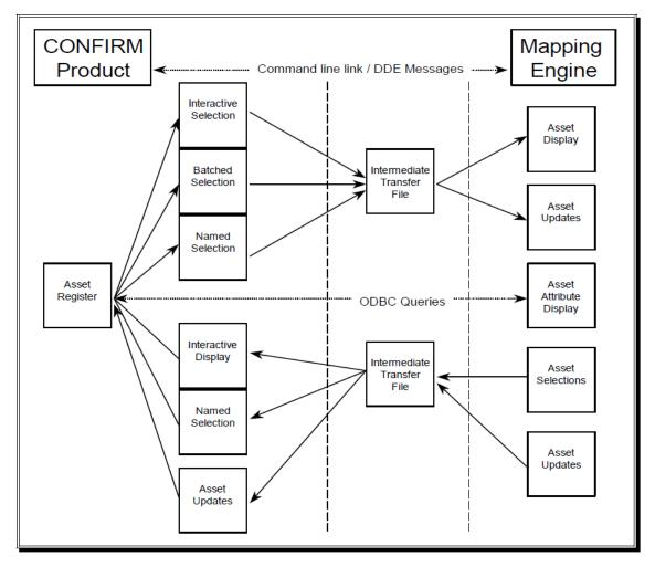
The interface is generally achieved by one of two methods. The first involves either the Confirm system or the GIS acting as a client or server application to each other passing details of asset selections for further processing using a combination of Dynamic Data Exchange (DDE), or Command Line Parameters, and intermediate transfer files.
