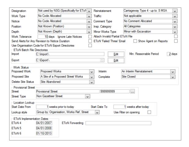
The following fields will set default entries for Street Work form when an electronic Notice cannot be read for these fields: Designation, Work Type, Notice, Position, Depth, Traffic and Minor Works Type. In each field, select from the drop down list. The drop down lists reference the Lookups of the same name in each case. (Designation Lookups are held in the **Street Register\Street Lookups**\Gazetteer Lookups. All the other Lookups are found in **Street Works Lookups** on page 239)
