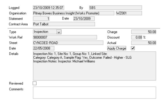
When the Type is Inspection, the Statement Item screen contains an additional 'Apply Charge' field. This will be checked by default for the primary Site and unchecked by default for Linked Sites.
