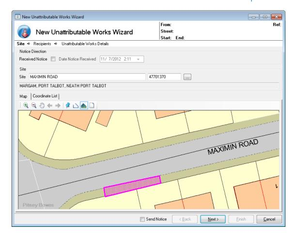
The Wizard will prevent the User from progressing to the next step if a Provisional Street has been selected (as determined by the Streets Record Type and the Provisional Street Type specified in the **Street Works System Settings**).
