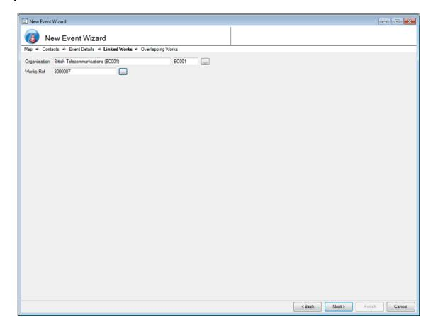
If the Works Type selected on Event Details step is one with a Classification of Notifiable Works then the Linked Works step is displayed. This step will be skipped if the Works Type does not have a Classification of Notifiable Works. The Linked Works step optionally allows an Event to be linked to a Street Works, which then provides a guick method of navigating between them.
