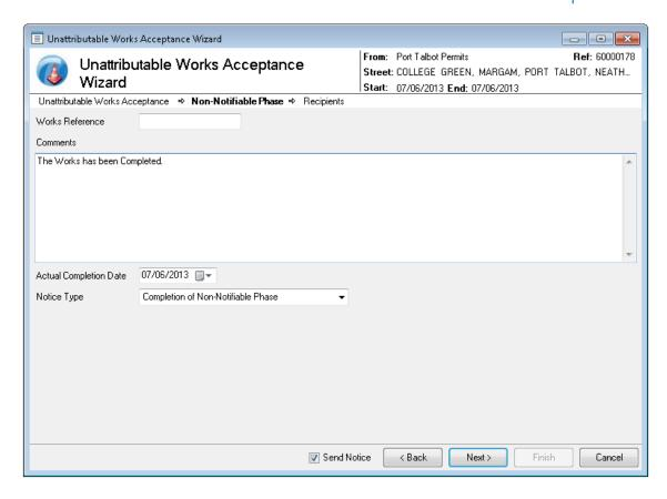
Work Reference: Supply a reference for the Works being entered. The combination of Organisation Code and Works Reference must be unique and can only contain uppercase letters A-Z, numbers 0-9 and the / and - separators. If invalid characters are entered, this message will occur when the 'Next' button is clicked.
