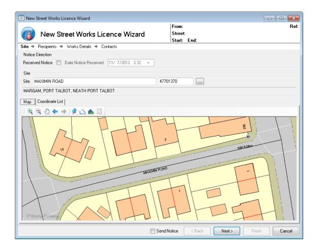
The Wizard will prevent the User from progressing to the next step if a Provisional Street has been selected (as determined by the Streets Record Type and the Provisional Street Type specified in the **Street Works System Settings**).
