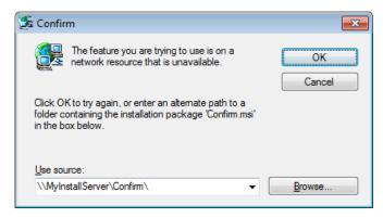
This is caused by the uninstallation of the previous version, which now occurs as part of the upgrade process. Pre v14 installers try to access their original installation media during this uninstall stage. The user can click '**Cancel**' and ignore this message each time it appears without impacting the upgrade process. From v14, installers do not try to access the original installer during uninstall, avoiding this issue moving forward.
